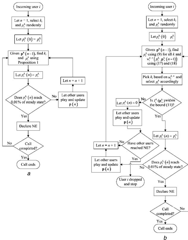
**Figure 2** Flow chart illustrating the NCPG and the NCPGL algorithms
