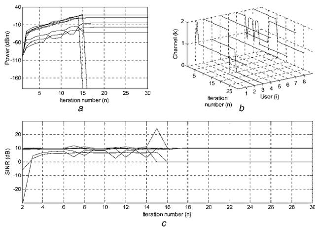
**Figure 5** Convergence of the NCPGL in an infeasible system for  $N = 8$  and  $K = 2$
