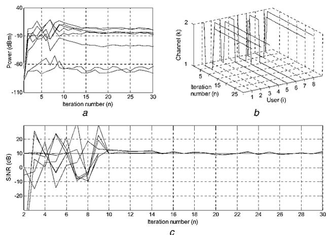
**Figure 3** Convergence of the NCPG in a feasible system for  $N = 8$  and  $K = 2$
