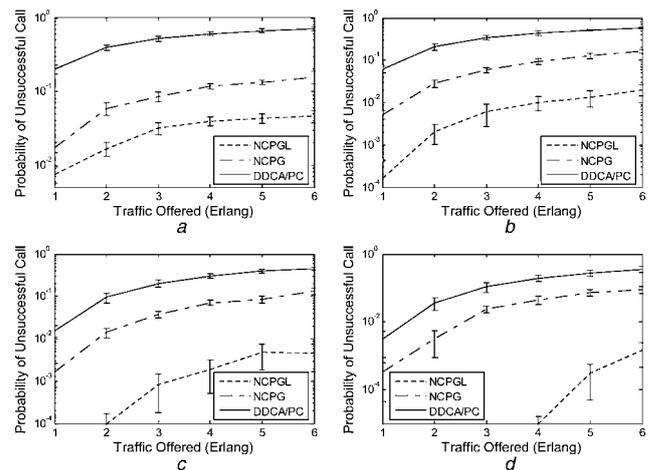
**Figure 7** Probability of unsuccessful call against traffic offered for the NCPGL, the NCPG and the DDCA/PC in different systems with  $K = 2, 3, 4$  and 5
