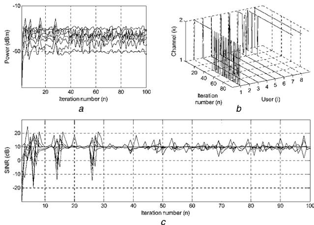
**Figure 4** Divergence of the NCPG in an infeasible system for  $N = 8$  and  $K = 2$
