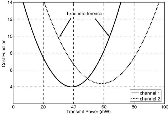
**Figure 1** Cost function against users' transmission power under fixed interference on two different channels
